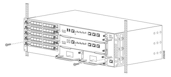
Figure 3-4 Installing the Chassis to support the Japanese JIS Rack Standard
